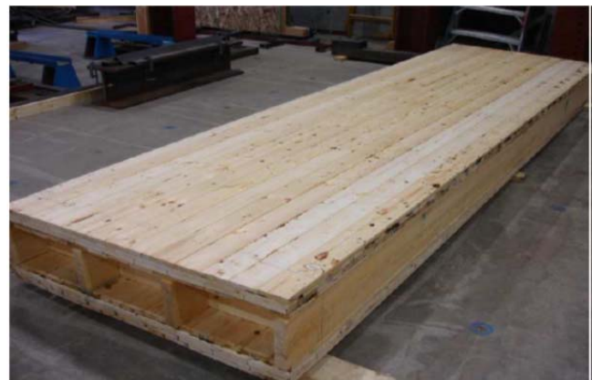
Figure 3 – A box system consisting of 45° laminated plates.
