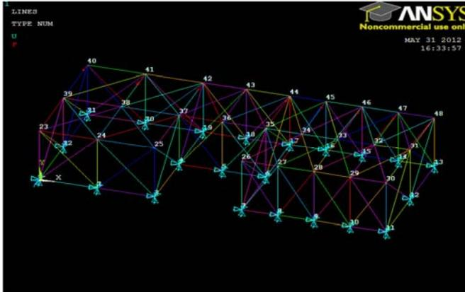
The results from the detailed numerical model were used to determine an average shear modulus value,  $G$ , which in turn was employed to calibrate the axial stiffness,  $EA$ , of the members of the simplified truss model shown in this figure. This facilitated the analysis of shear wall forces in a large building. A variety of diaphragm and shear wall stiffness values were explored to seek an understanding of the influence of in-plane stiffness on the shear-wall-force distribution.
