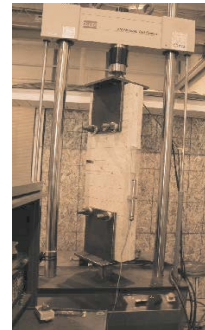
Figure 2 - CLT-to CLT connection test
