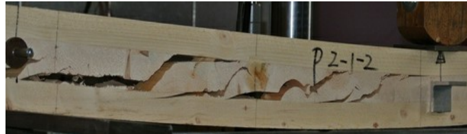
Figure 3 Failure mode of 3-layer CLT beam under bending test
