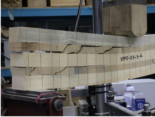
Figure 6: Failure mode in the ramp loading test
