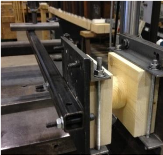
Figure 3: Test setup of torsional shear test
