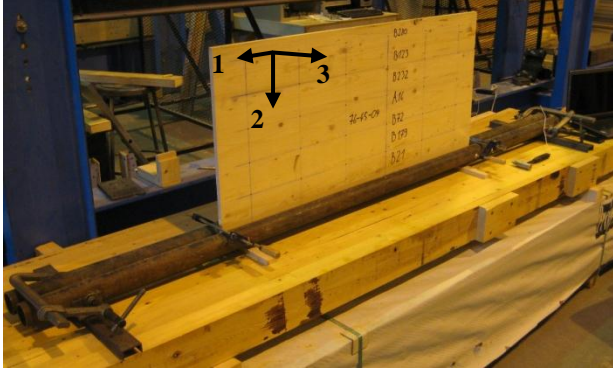
Figure 1: Test setup for modal tests in FFFS BCs
