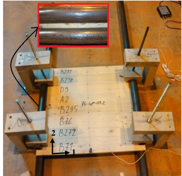
Figure 4: Test setup and clamping detail for SFSF test
