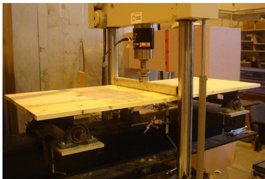
Figure 4: Bending test setup for E_{11} value evaluation
