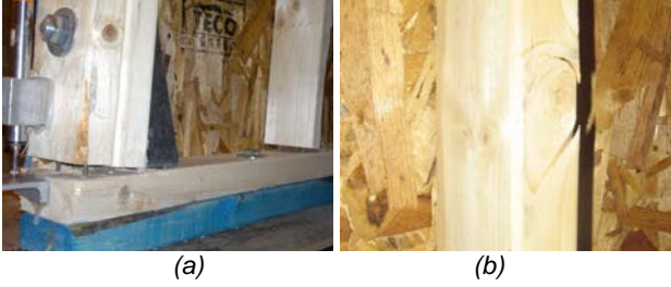
Figure 4: Failure modes of shearwalls sheathed with OSB
