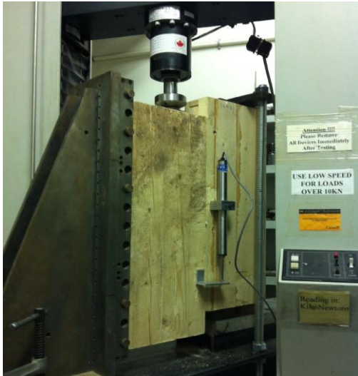
Figure 5: Shear test apparatus
