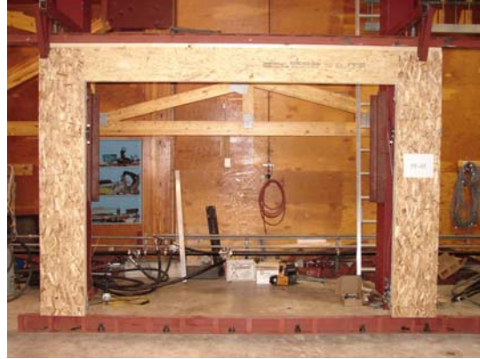
Figure 2: Test setup of the portal frame
