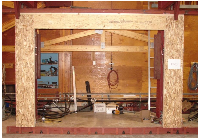
Figure 1: Test setup of the portal frame wall assembly
