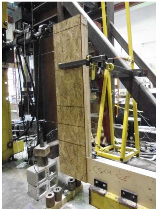
Figure 3: Test set-up with MIDPLY portal frame corner specimen installed
