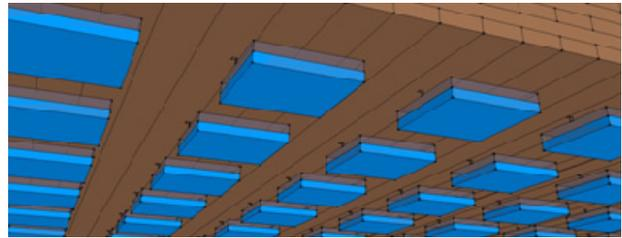
**Figure 3:** DLDs attached to CLT floor bottom
