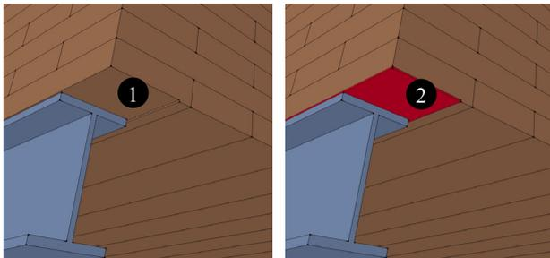
**Figure 2:** Notch cut ①, and damping layer inserted ②
