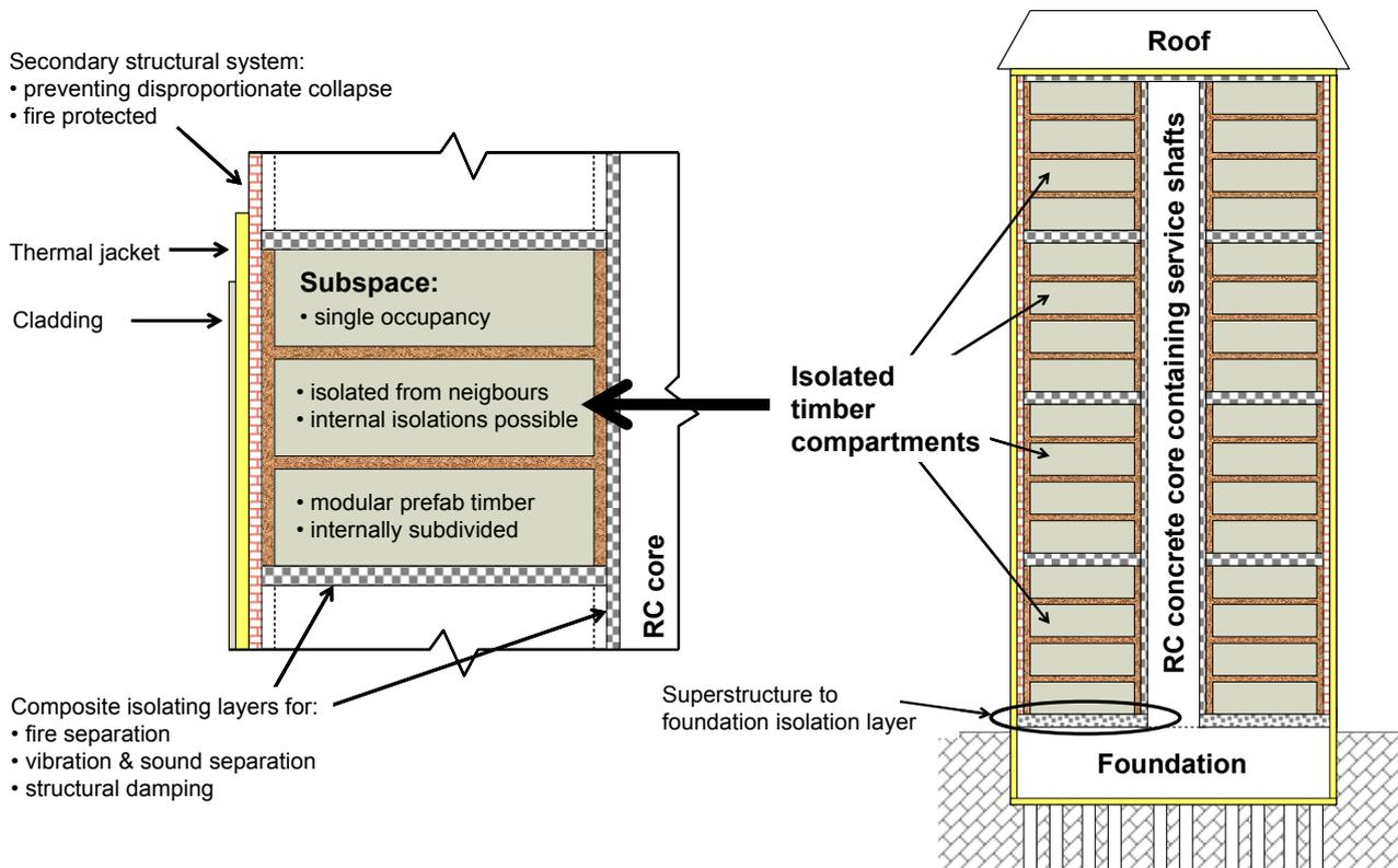
Figure 1: High-rise building with isolated timber compartments. Isolation to be defined [1].
