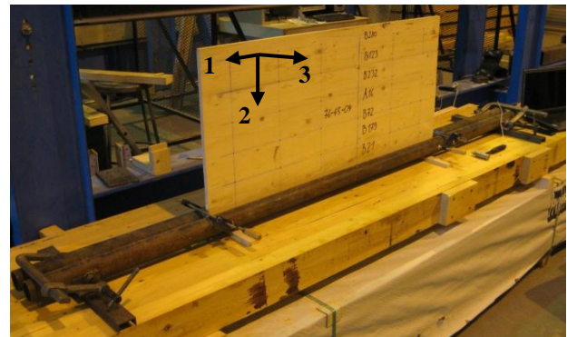
Figure 1: Test setup for modal tests by [3]
