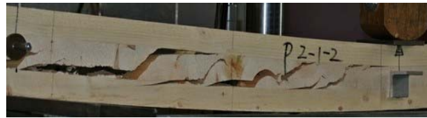
Fig.5 Failure mode of 3-layer CLT beam under bending test
