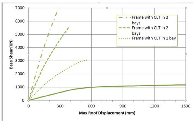
Figure 3: Pushover Curve comparison between frames with CLT infill walls at 6 storeys
