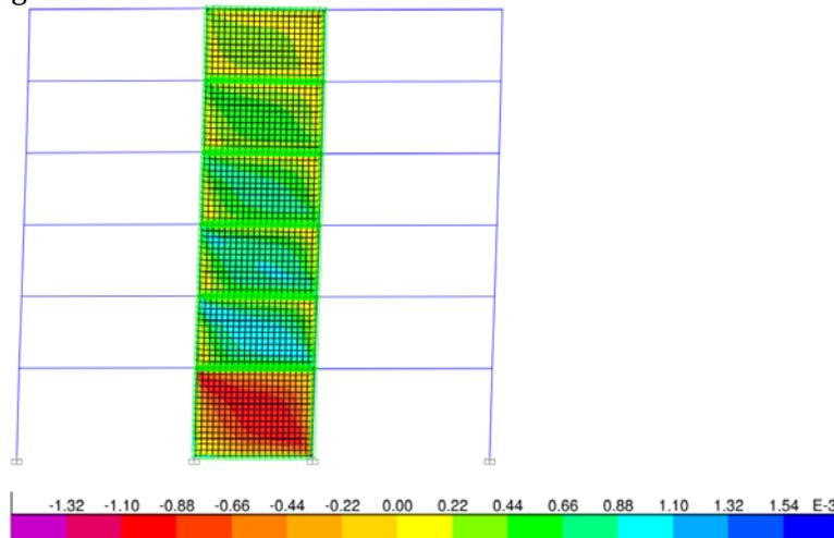
Figure 2: Deflected steel moment frame with infill wood shear walls with panel shear
