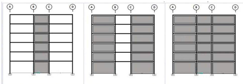
1. Figure 1: Wall Locations for Frame with Infill wall locations
