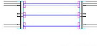
Figure 3 The cross section of the triple-leaf wall in the filler wall
