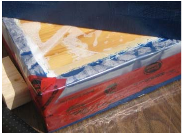
Fig. 13. Condensation on Interior of Polyethylene Sheet for Low Interior Permeance Panels
