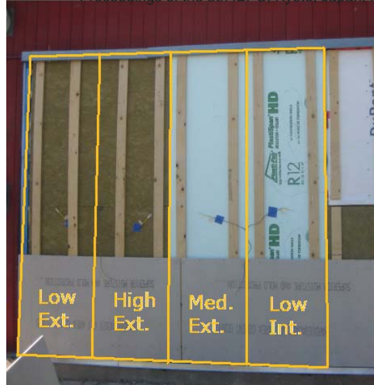
Fig. 7. CLT test wall with insulation, strapping and cladding.
