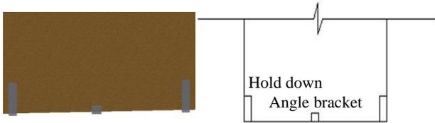
Figure 2: Configurations of hold downs and angle brackets
