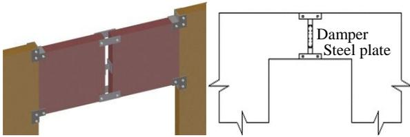
Figure 3: Configurations of dampers
