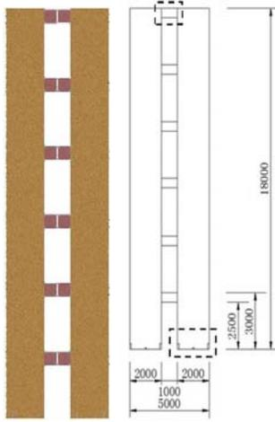
Figure 1: Elevation of the shear wall with coupling beams
