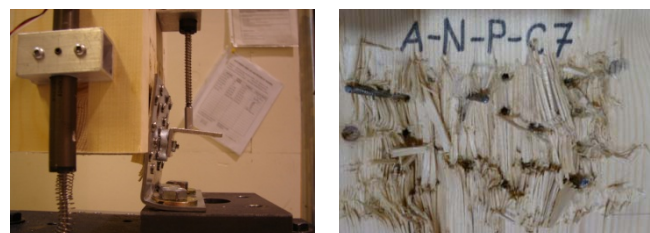
Figure 2: (a) off-centred fastened bracket, (b) damaged CLT panel after cyclic loading protocol
