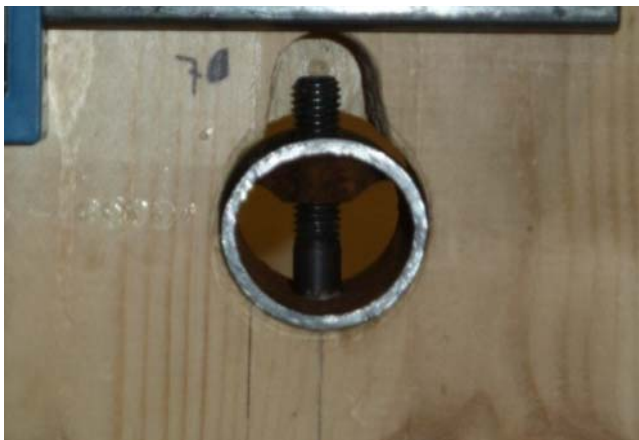
Figure 4: Plastic deformation of the tube under monotonic loading protocol
