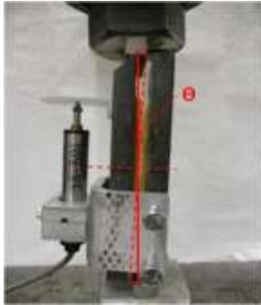
Figure 1: Experimental set-up for 2-plate shear test
