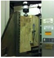
Figure 1: Shear test apparatus
