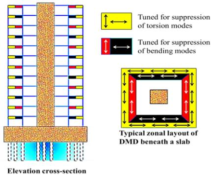
**Figure 1:** Zonal placement of tuning of damper arrays in DMD system (courtesy of Advanced Construction Technologies III)
