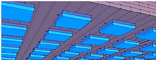
**Figure 2:** DMD array on undersides of CLT floor slab (adapted from Weckendorf and Smith)
