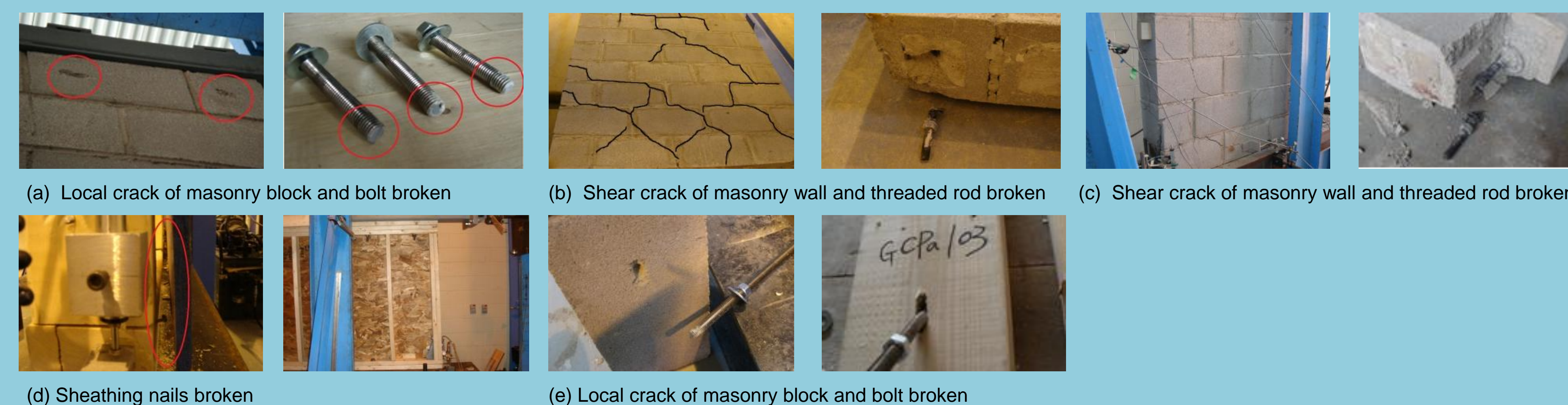
Figure 5: Failure mode of test specimen: (a) HW1; (b) HW2; (c) two-storey masonry wall; (d) one-storey wood wall; (e) wood-masonry connection
